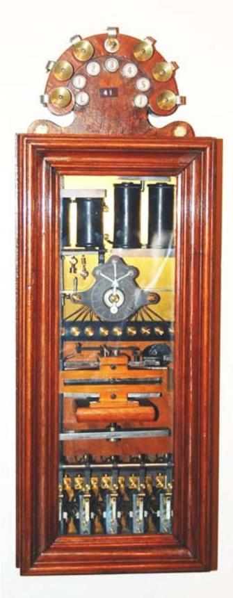
This switch can connect one exchange line to five subscriber lines. The subscribers have to be located near to the switch, preferably in the same building. The subscribers can not call to each other. Only one of the subscribers can at a time have the exchange line. The others are then off. This equipment is very rare and besides this specific object is in unusual good condition.
