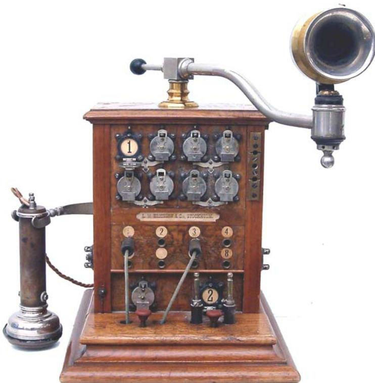
This small telephone exchange for 8 lines is the most valuable item in Museum. The instrument exist in the oldest LME catalog 1886 and is today as far as we know the only one in the world. The model year of the equipment is 1881, but it had then a helical microphone. The museum exchange has a more stable carbon microphone.
