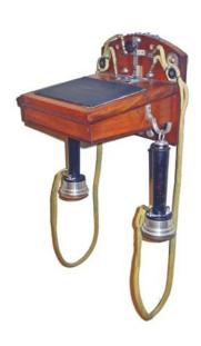
by Reiner. There is a receiver for both ears, which made the listening easier. You can not see any microphone, because the writing surface is the membrane of the microphone. Under the surface there are the magnet and coils of microphone. Both this microphone and the use of two earpieces are Adérs inventions.
