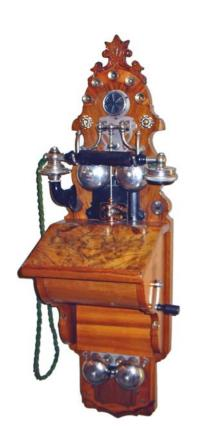
Basically the same telephone as the previous but with out of the ordinary design. The back plate, the bell system cover and the pulpit are from old LME model 301. The other parts are from CK 550. The timberwork is especially fine. The material is stained oak, not walnut as in general. This telephone is not from LME factory. The maker has been some skilled craftsman. The phone is also for sure an unique article.
